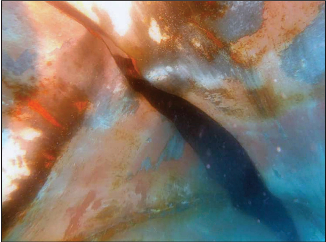
Figure 7: Split in shell plating between frames 169 and 178
