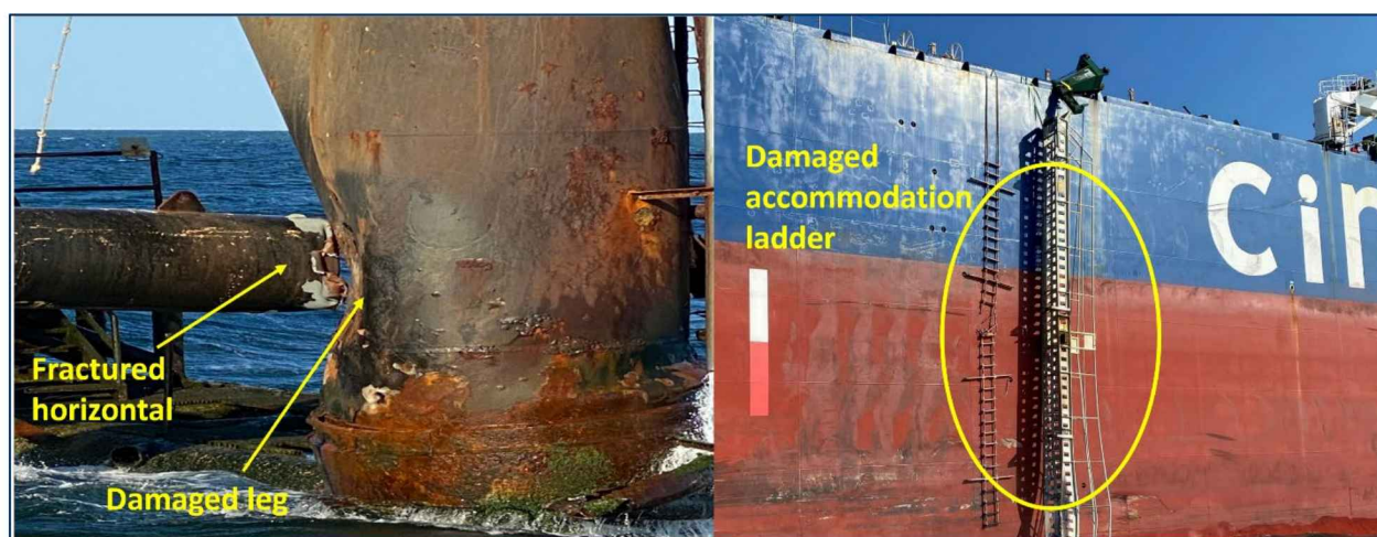
Figure 5. Damage to SP-57B (left) and Atina (right). (Source: Coast Guard)
