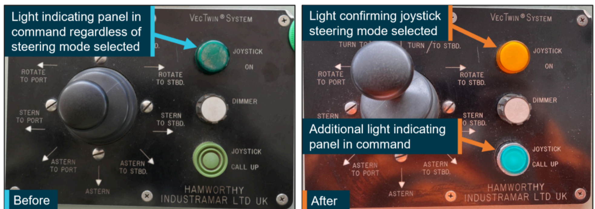
Figure 13: Joystick panel at the time of the accident (left) and after modifications (right)
